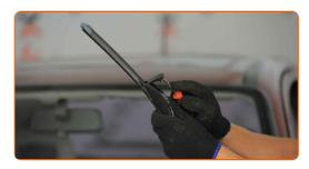
Remove the blade from the wiper arm.
