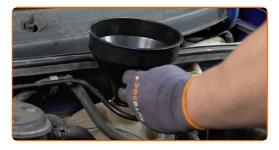
Pour coolant in the coolant reservoir.
