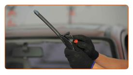
Remove the blade from the wiper arm.
