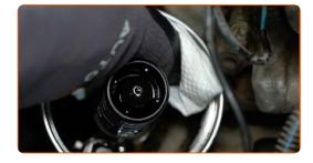
Install the cover of the oil filter housing and screw it on. Use a drive socket #32. Use a torque wrench. Tighten it to 15 Nm torque.
