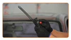
Remove the blade from the wiper arm.
