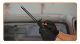
Remove the blade from the wiper arm.
