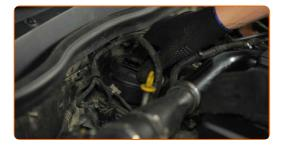
Remove the fuel filter cover with the old filter cartridge attached.
