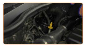
Attach the pipe to the fuel filter.
