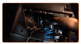
10 Install the cabin filter to its mounting seat.
