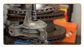
Screw the new engine mount to the bracket. Use Torx T55. Use a ratchet wrench.
