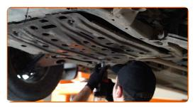
Remove the hydraulic transmission jack.
