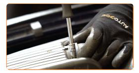
Remove the fender protection cover.
