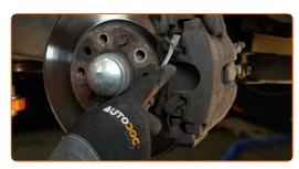
11 Remove the brake caliper.
