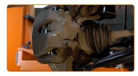
20 Install the brake caliper retaining spring.
