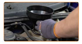
Pour coolant in the coolant reservoir.
