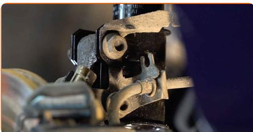
**37** Secure the stabilizer link on the suspension strut. Use a combination spanner #19. Use a drive socket #18. Use a torque wrench. Tighten it to 65 Nm torque.
