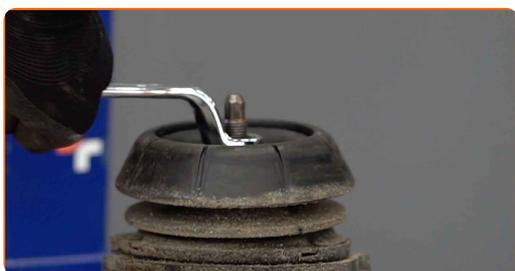
**23** Remove the shock absorber mount, boot and bump stop. Use a crowbar.
