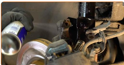
**31** Fix the shock absorber strut on the steering knuckle.
