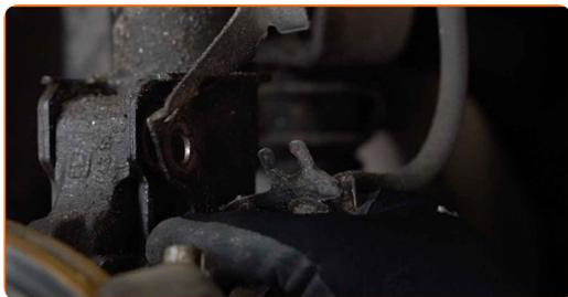
**17** Disconnect the steering knuckle from the shock absorber strut. Use a crowbar.
