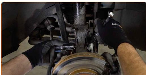
**14** Prop up the steering knuckle. Use a hydraulic transmission jack.
