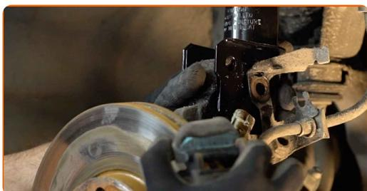
**32** Install the new steering knuckle bolts.
