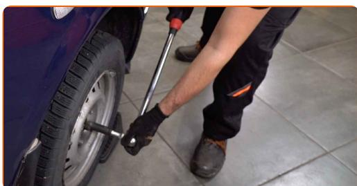
**42** Tighten the shock strut top mount. Use a drive socket #17. Use a torque wrench. Tighten it to 50 Nm torque.
