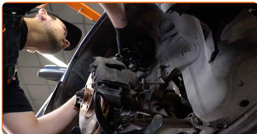
**29** Tighten the upper fastening nut of the shock absorber strut. Do not tighten it.
