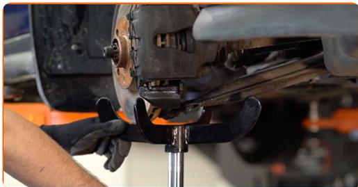
**15** Remove the fastener attaching the brake hose to the shock strut.
