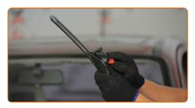
Remove the blade from the wiper arm.
