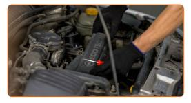
5 Detach the connector from the ignition coil. Use a flat screwdriver.
