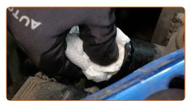
Clean the thermostat housing. Use a wire brush. Use all-purpose cleaning spray.
