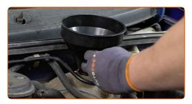
Pour coolant in the coolant reservoir.
