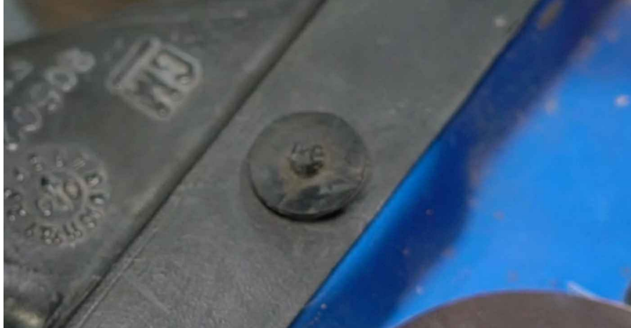
33 Remove the coolant reservoir cap.
