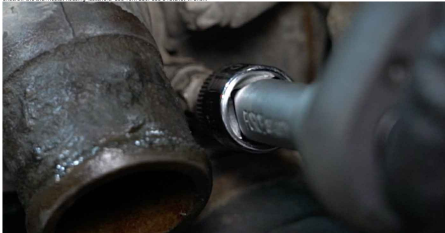
21 Remove the thermostat housing together with the thermostat.
