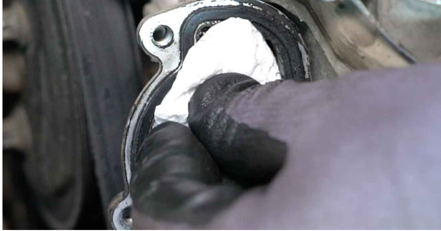
23 Remove the rubber strip.
