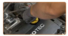
Clean the oil filter housing cap. Use all-purpose cleaning spray.
