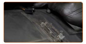
7 Unscrew the fasteners of the air distribution housing assembly. Use a drive socket #10.
