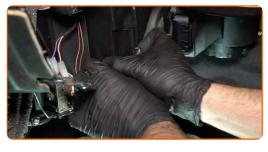
Reinstall the air distribution housing assembly.
