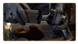
Remove the oil filter cover O-ring. Use a flat screwdriver.
