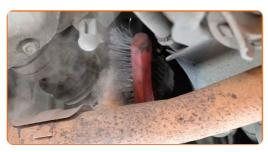
Detach the oxygen sensor connector.
