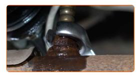
Remove the oxygen sensor.
