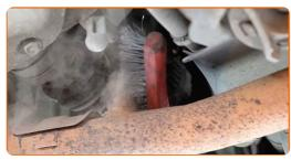
Detach the oxygen sensor connector.
