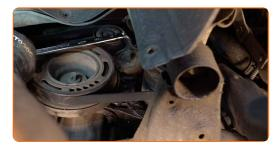
Return the tensioner pulley to its initial position.
