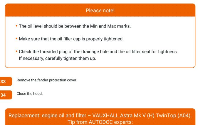
• Note that oil pressure warning light, which indicates insufficient pressure in the lubrication system, may be on for a longer time than usual. After a few seconds, the oil will fill all the channels, and the light will go out.
