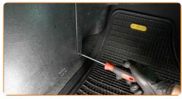
Remove the clips of the bottom trim panel. Use a clip removal tool.
