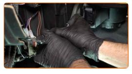
Reinstall the air distribution housing assembly.
