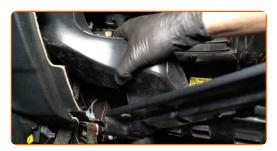
Release the cabin filter cover clips. Use a clip removal tool.
