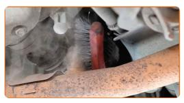
Detach the oxygen sensor connector.
