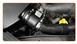
6 Remove the air intake pipe.
