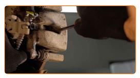
Remove the brake caliper. Use a crowbar.
