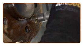
Remove the brake disc.
