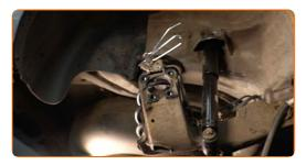
Remove the brake disc cover.
