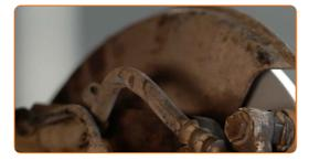
Clean dirt from the brake hose bolt. Use a wire brush. Use a brake cleaner.
