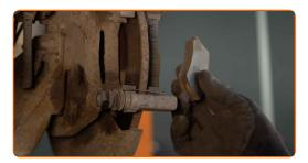
Clean the brake caliper bracket fasteners. Use a wire brush. Use a brake cleaner.
