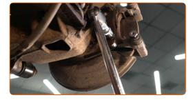
18 Remove the caliper bracket.
