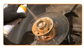
41 Install the brake disc.
