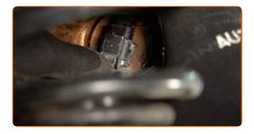
Connect the ABS sensor wiring.
