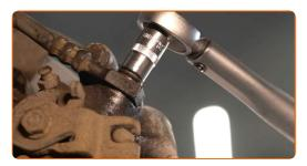
Remove the brake hose clamp.
