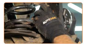
Tighten the wheel hub bearing fasteners. Use a drive socket #16. Use a ratchet wrench.
