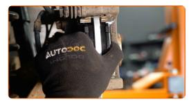
Install the brake caliper and fix it.
