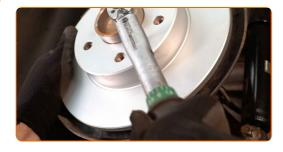
Install the brake caliper bracket.
