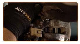
Tighten the brake hose fastener. Use a drive socket #11. Use a torque wrench. Tighten it to 40 Nm torque.
