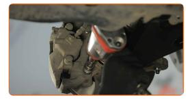
Install the mounting bracket of the brake hose and the ABS cable.
