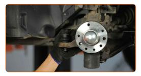
Tighten the fastening nut connecting the tie rod end to the steering knuckle. Use a drive socket #19. Use a torque wrench. Tighten it to 30 Nm torque.+90°
