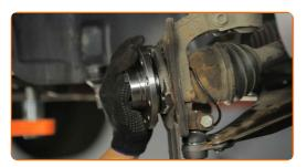
Tighten the wheel hub bolts. Use a drive socket #E18. Use a torque wrench. Tighten it to 90 Nm torque.+45°
