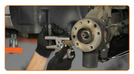
Unscrew the wheel hub bolts. Use a drive socket #E18. Use a ratchet wrench.
