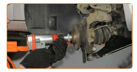
Remove the drive shaft from the wheel hub. Use a rubber mallet.
