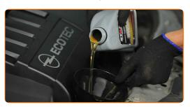
Replacement: engine oil and filter – VAUXHALL Astra Mk V (H) Estate (A04).
