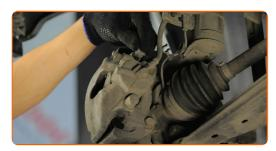
Install the brake caliper retaining spring. Use a flat screwdriver. Use pliers.
