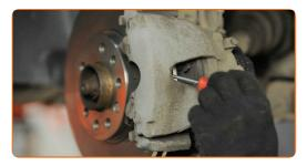
Remove the brake caliper.
