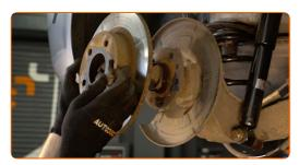
Replacement: wheel bearing – VAUXHALL Astra Mk V (H) (A04) Hatchback. Tip from AUTODOC:
