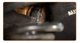
Connect the ABS sensor wiring.
