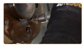
Remove the brake disc.
