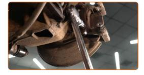
18 Remove the caliper bracket.
