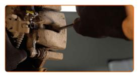
Remove the brake caliper. Use a crowbar.
