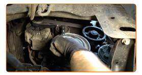
Return the tensioner pulley to its initial position. Use a combination spanner #15.
