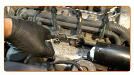
Tighten the glow plugs. Use the spark plug socket #8. Use a torque wrench. Tighten it to 10 nm torque.
