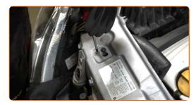
Remove the air distribution housing assembly.
