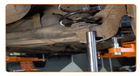
Tighten the top shock absorber fastening. Use a drive socket #E20. Use a torque wrench. Tighten it to 90 Nm torque.
