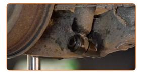
Unscrew the upper fastener of the shock absorber. Use a drive socket #E20. Use a tap wrench.
