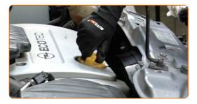
Tighten the oil filler cap.
