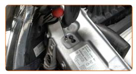
Remove the air distribution housing assembly.
