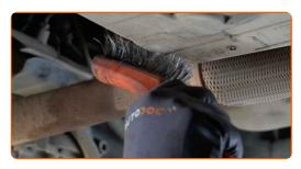
Unscrew the drain plug. Use Torx T45. Use a ratchet wrench.
