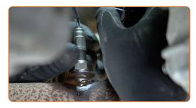
Tighten the oxygen sensor fastener. Use a drive socket #22. Use a torque wrench. Tighten it to 31 Nm torque.
