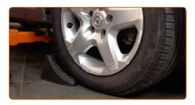
Loosen the wheel mounting bolts. Use wheel impact socket #17.
