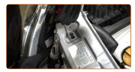
Remove the air distribution housing assembly.
