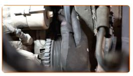
6 Return the tensioner pulley to its initial position.
