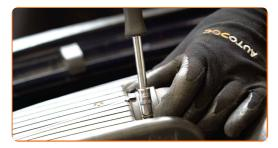
Remove the fender protection cover.
