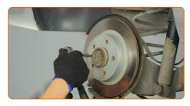
13 Remove the brake disc.
