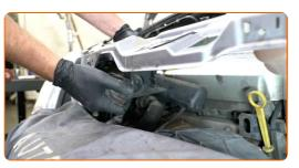
Replacement: engine thermostat – VAUXHALL Astra Mk IV (G) Convertible (T98). Tip:
