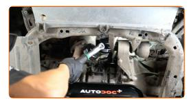
Replacement: engine oil and filter – VAUXHALL Astra Mk IV (G) Convertible (T98). Tip:
