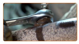
Remove the oxygen sensor.
