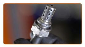
10 Install the new oxygen sensor.
