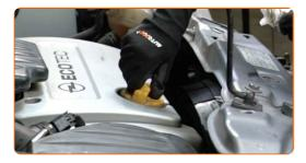
Tighten the oil filler cap.
