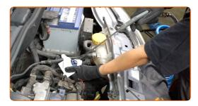
Plug in the ignition coil connector. Make sure you hear a click indicating that it is locked in place.
