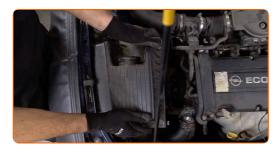
Unscrew the filter housing fastening bolts. Use Torx T30. Use a ratchet wrench.
