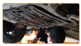
Remove the hydraulic transmission jack.
